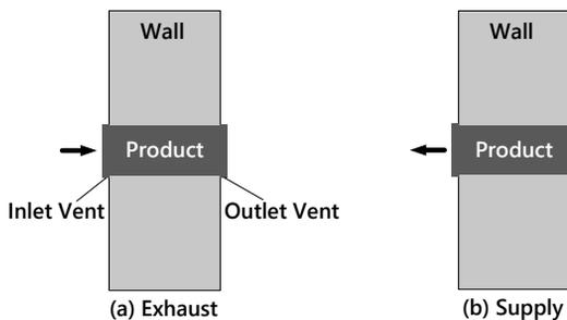
**Figure 1.** Schematic of the installation of the product in (a) exhaust and (b) supply modes.
